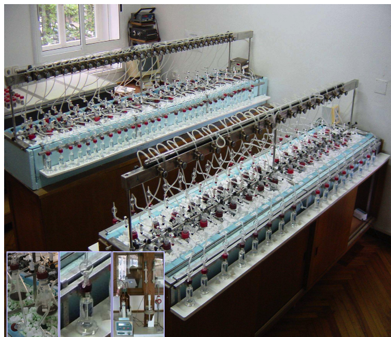
Fig. 2. Respirometric system used to perform the soil incubation experiments.
