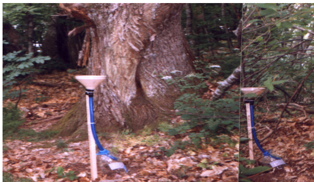
Fig. 3. Permanently open collectors for the deposition of heavy metals.
