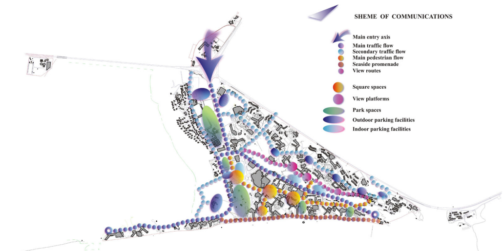
Fig. 4. Scheme of communications.
