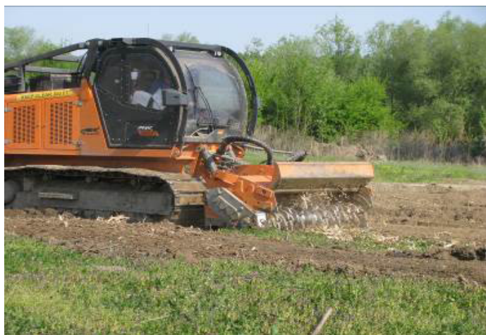
Fig. 2. Specialized milling unit Prime Mover PT-400 with multifunctional forest tiller FAE 300/S, subsection 13 e in State Forestry Service „Oryahovo“.
