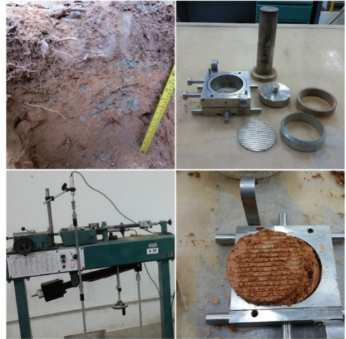
Fig. 2. The process of undisturbed soil sampling and analyzing with direct shear box machine.
