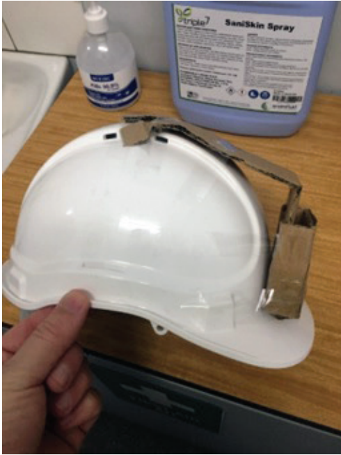
Fig. 1. DIY helmet mounted system (smart phone in use) – camera focusing set to 1 to 50 m.
